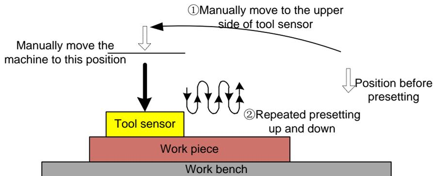
Fig. 3-24 The Process of Floating Presetting
