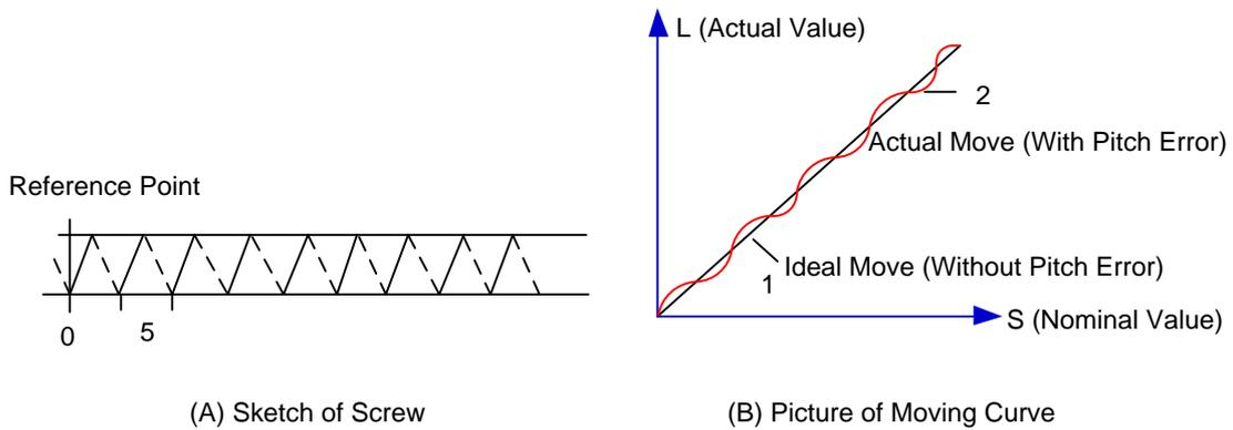
Fig. 3-37 Analysis of Pitch Error
