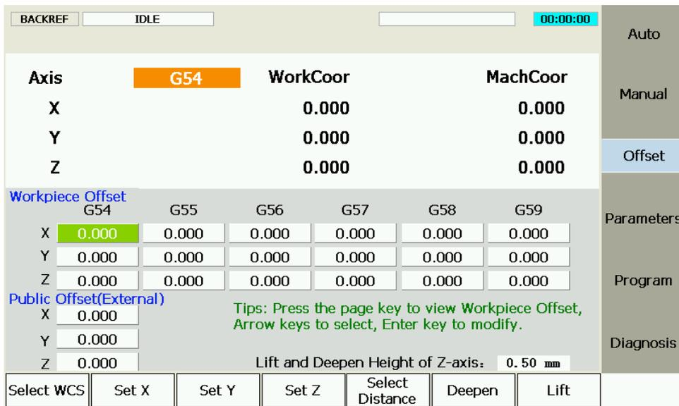
Fig. 3-32 [Offset] Function Section
