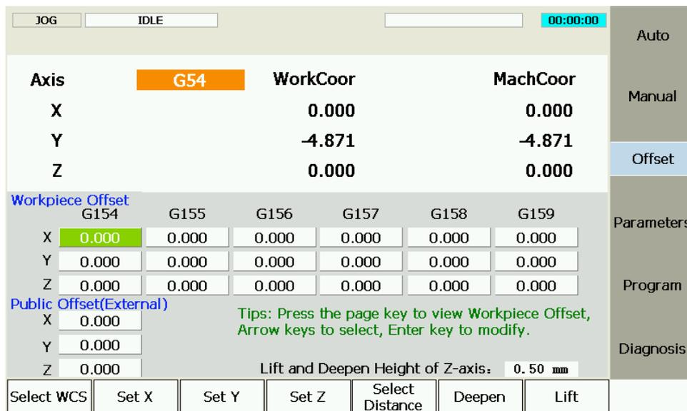
Fig. 3-31 Extended Coordinate System
