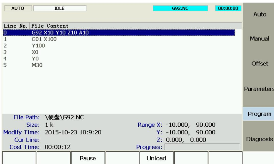
Fig. 3-54 Program File Interface (After loading a program)
