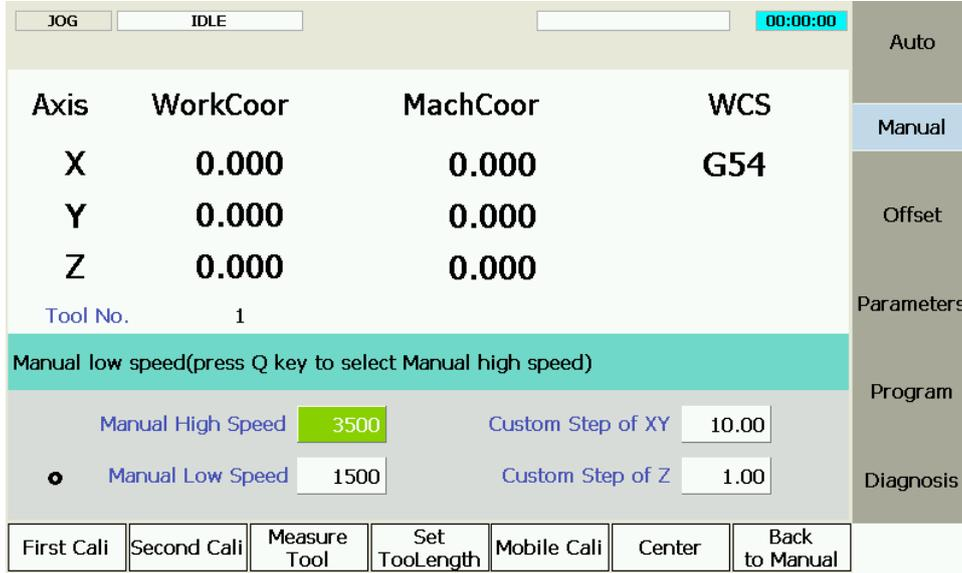
Fig. 3-23 Sub-screen of Tool Presetting
