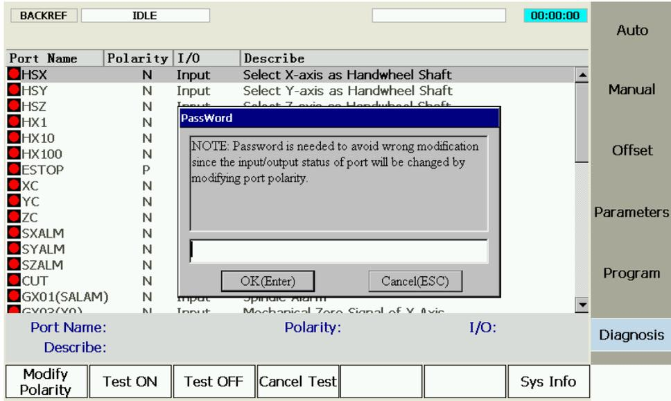
Fig. 3-4 Modify Polarity
