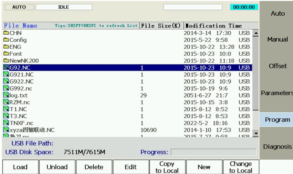
Fig. 3-53 Program File Interface (Before loading a program)
